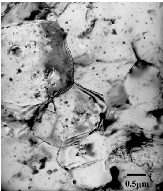
Figure 13 Micrograph showing small grains ( \sim 2 \mu\text{m} ) in a sample after 8 passes of warm ECAE ( 300^\circ\text{C} ) followed by a single room temperature pass.
